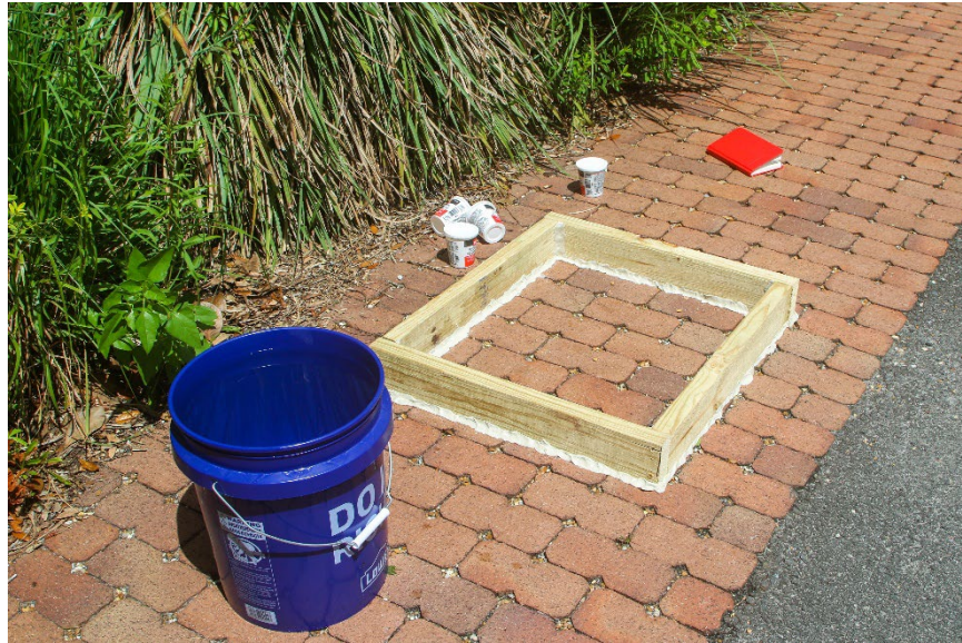
Figure 2. Simple Infiltration Test
