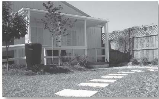
The Clemson Extension Carolina Yard constructed at the Charleston Exchange Park incorporates the use of pervious pavers, pervious walkways, a rain barrel, and a rain garden to educate the general public on the site-scale use of LID practices. Photo/USC
