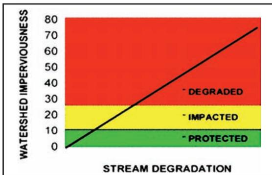
Figure 2.2.3.2a Relationship between imperviousness and receiving stream impact (adapted from Schueler, 1992).
