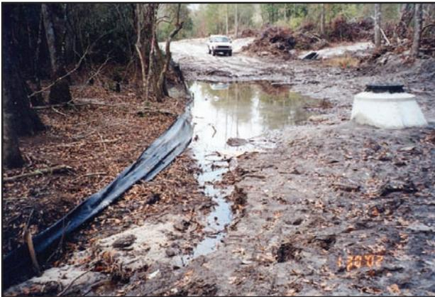
*Figure 2.2.2.2a Failed Sediment Control Fence*
