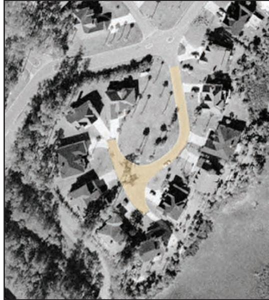
*Figure 2.3.3d T-Shaped Turnaround in Subdivision*
