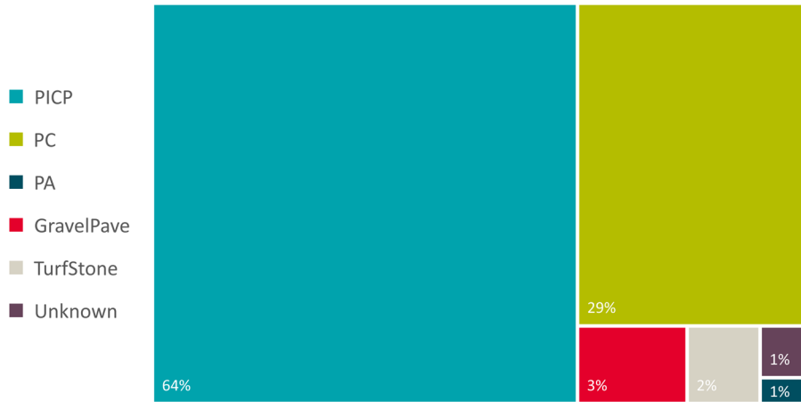
Figure 2. Types of Permeable Pavement (n=187 sites)
