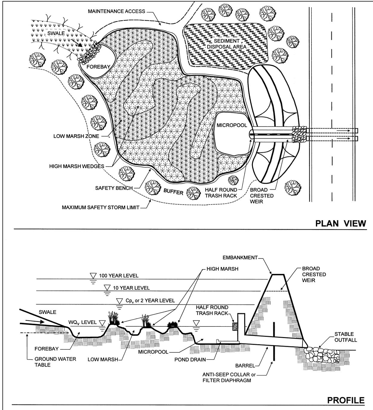
**Schematic of a Typical Pocket Wetland**
