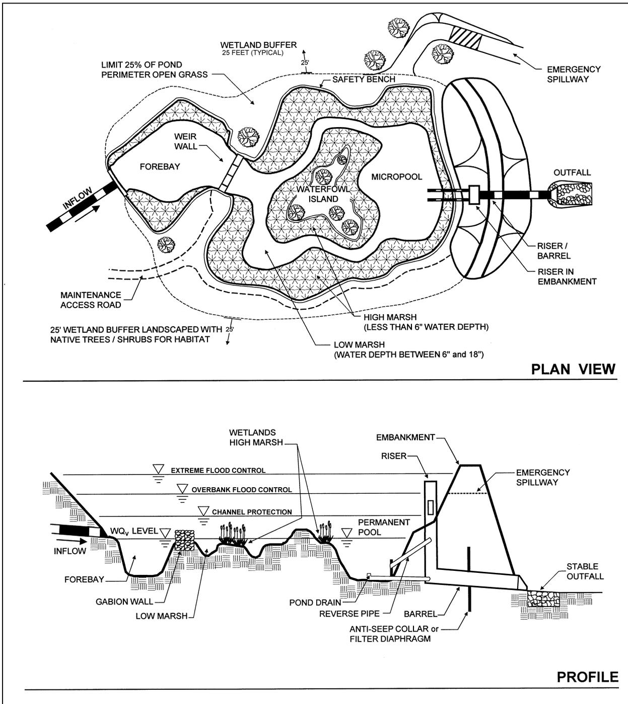
**Schematic of a Typical Shallow Wetland**
