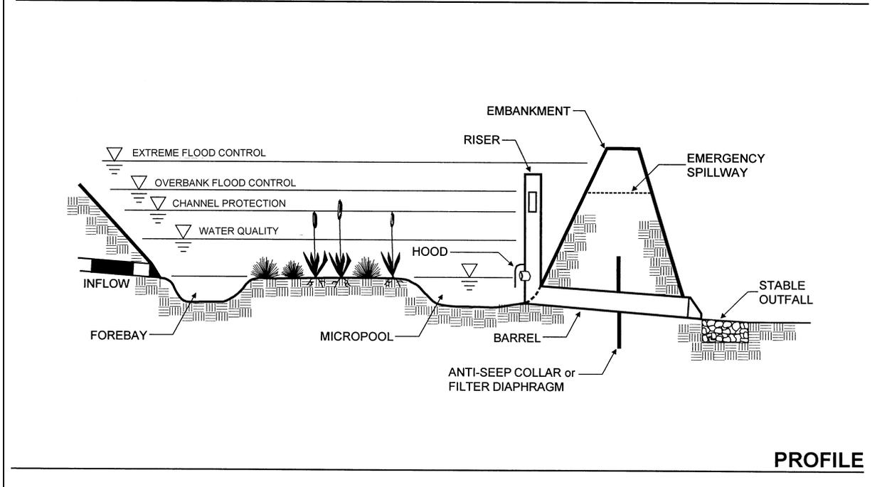
**Schematic of a Typical Micropool Extended Detention Pond**
