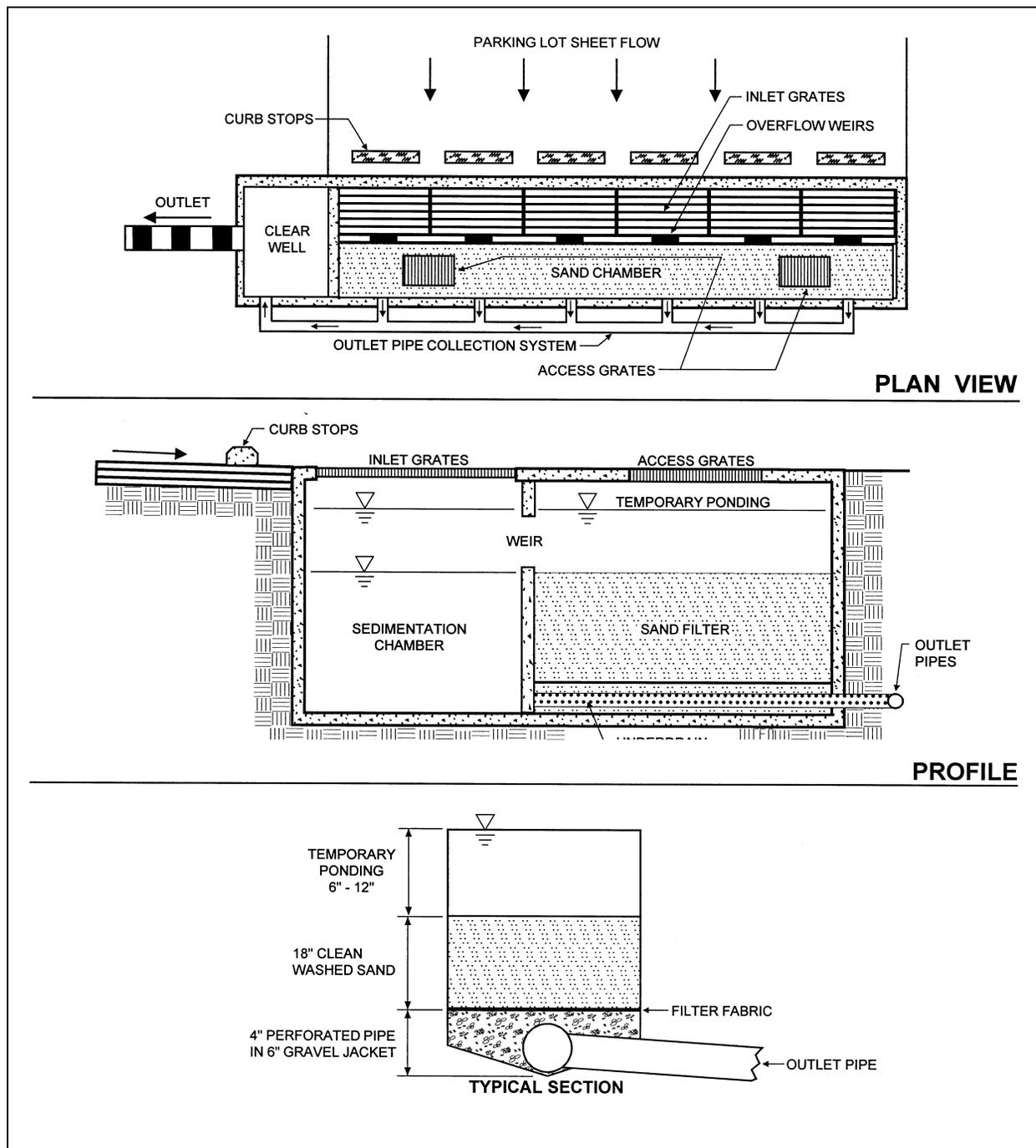
**Schematic of a Typical Perimeter Sand Filter**
