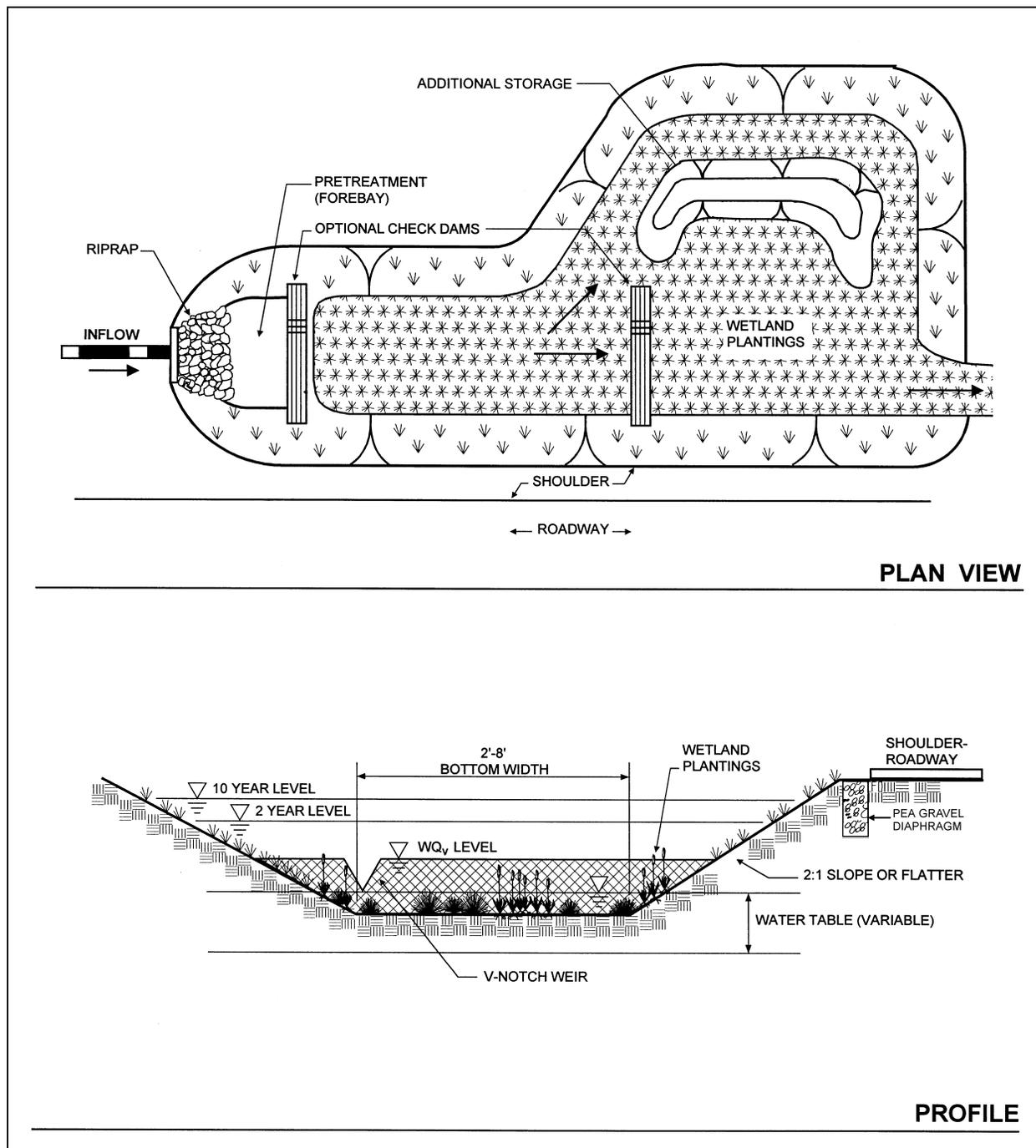
**Schematic of a Typical Wet Swale**
