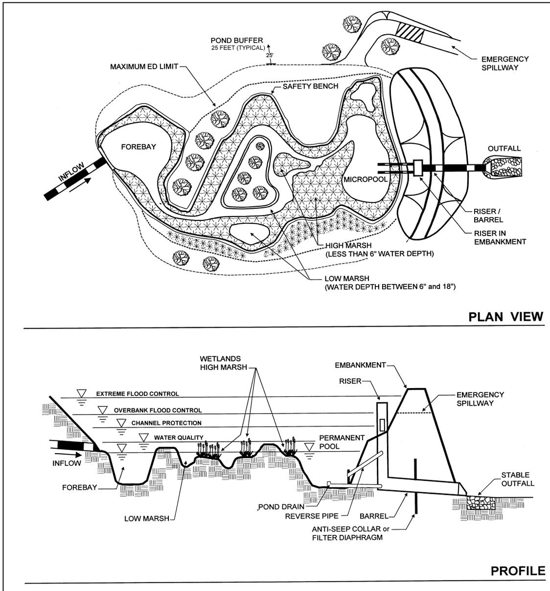
**Schematic of a Typical Shallow Extended Detention Wetland**
