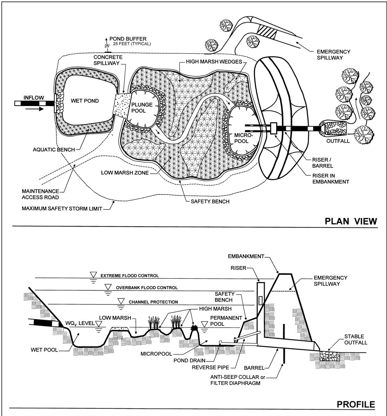
**Schematic of a Typical Pond/Wetland System**
