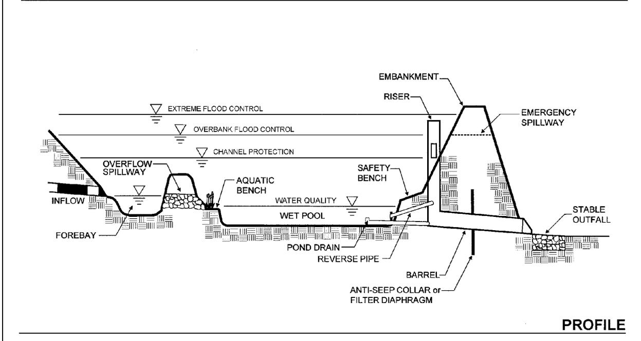
**Schematic of a Typical Wet Pond**
