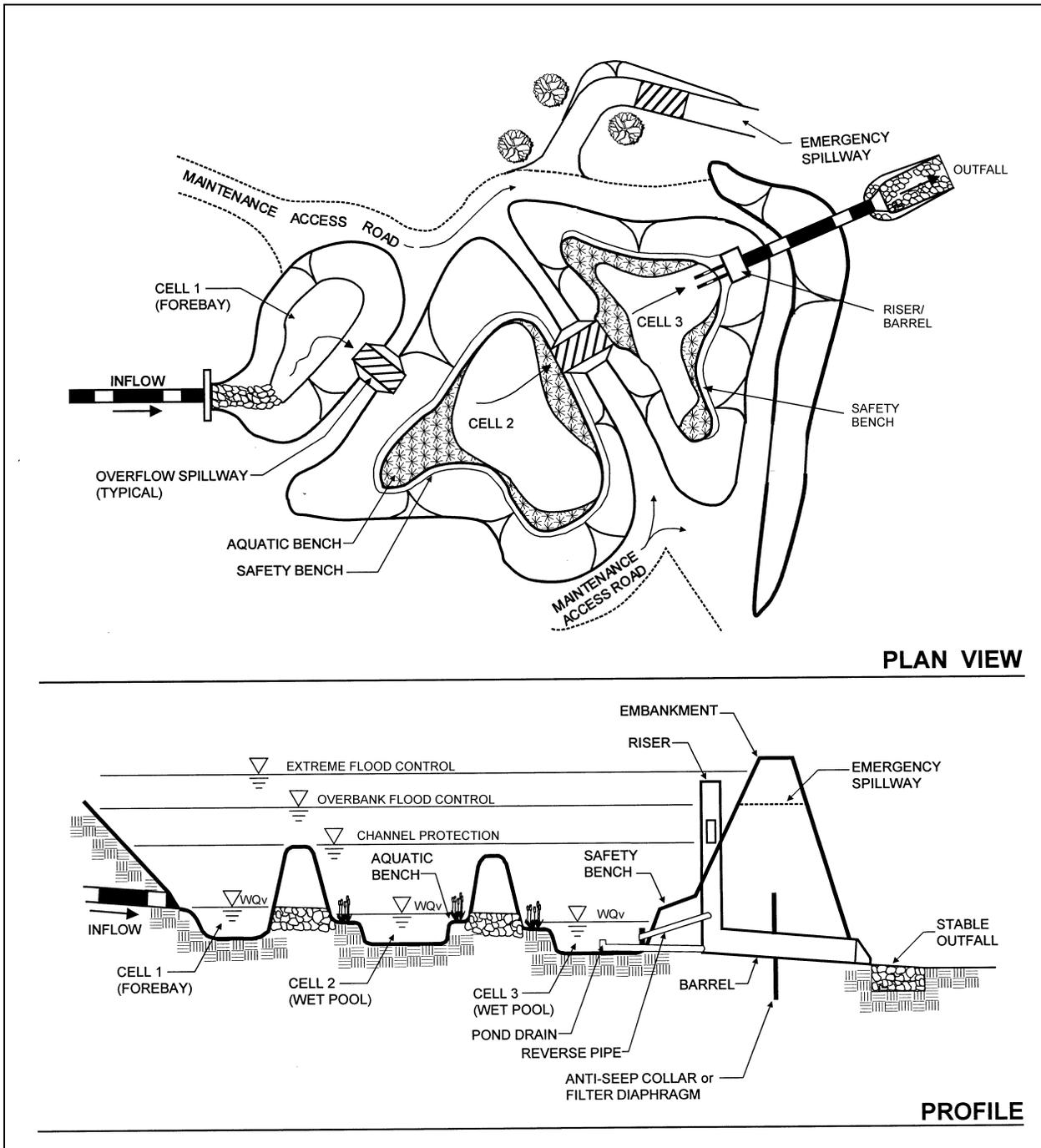
**Schematic of a Typical Multiple Pond System**
