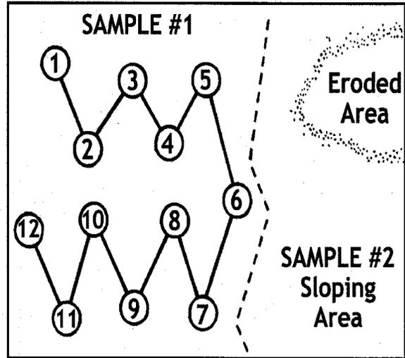
Figure 5. Zigzag pattern of soil sampling .
