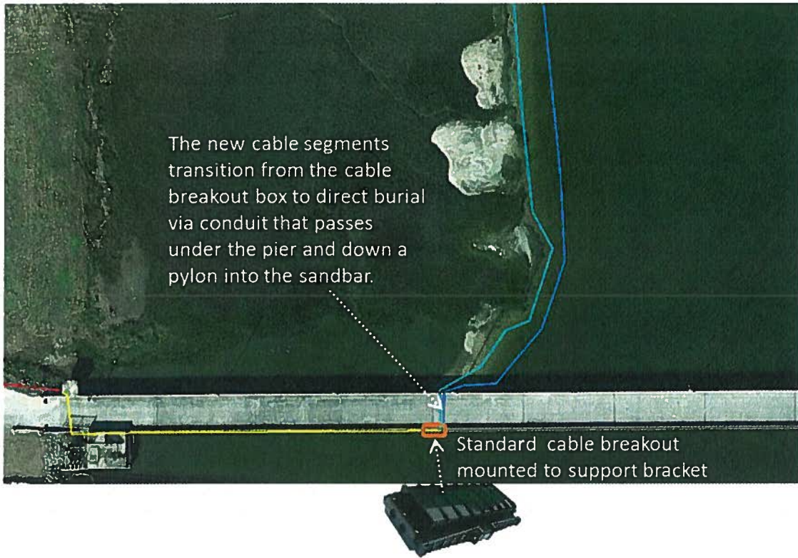
Figure 10. Transition from cable breakout to direct burial.
