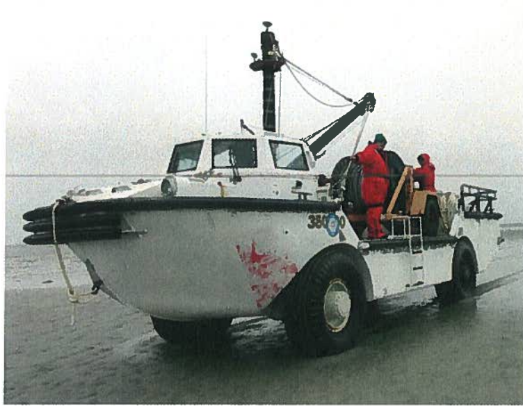
Figure 7. LARC amphibious vehicle to be used for the cable installation.
