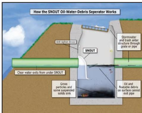
Figure 3.3.9c Illustration of a Snout Structure
