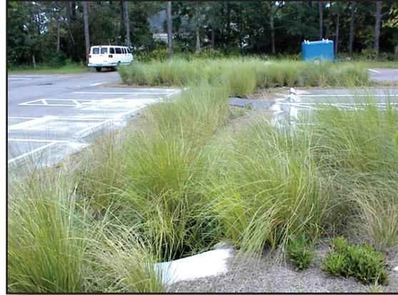
Figure 3.3.4c Bioretention Swales Using Wheelstops
