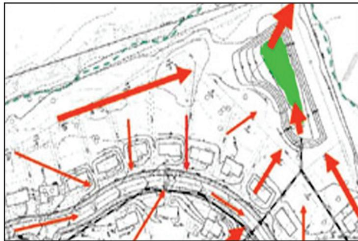
*Figure 3.1b Decentralized Approach: Manage Stormwater at source with LID Techniques*
