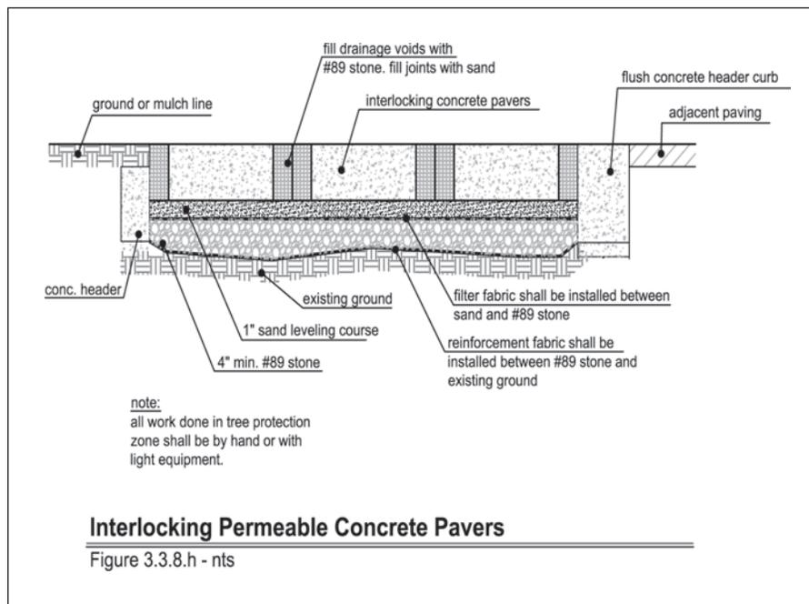
In addition to the relatively strict site constraints for porous pavement, a major limitation to the practice is the high failure rate some techniques have experienced in the field. According to EPA studies, 75% of porous pavement systems fail due to poor design, improper installation, use on soils with low permeability, traffic which exceeds the loading capacity and poor maintenance.
