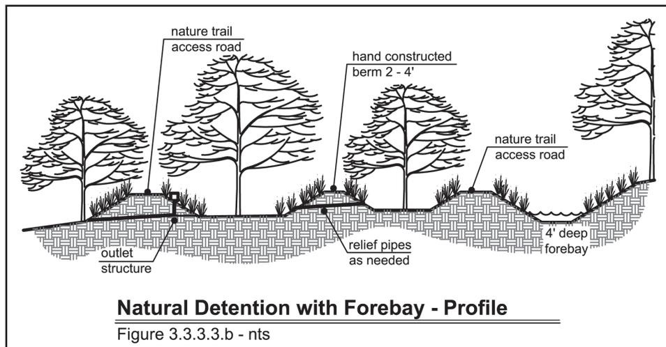
This is a practical, multi-functional solution for developments that must cross wetlands to access the buildable area of the tract. This practice creates a large green space area for the community, while detaining stormwater in the wetlands for infiltration and treatment by the soils and native vegetation. These natural detention areas can be installed with very little disturbance and require very little maintenance.
