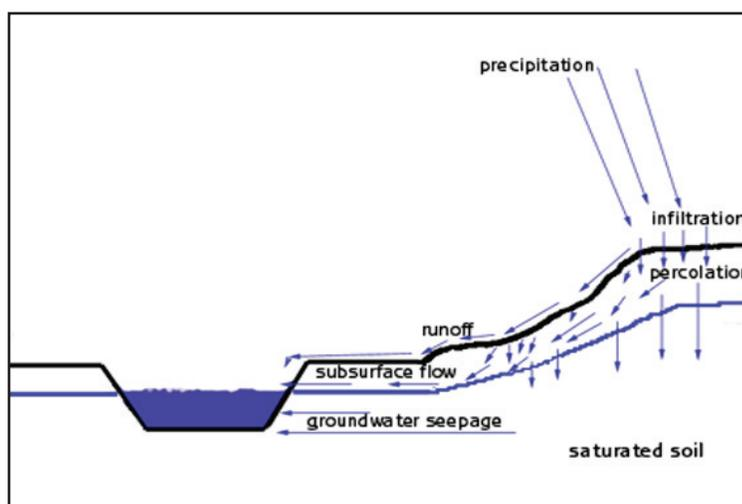
Figure 3.2.1a Illustration of Infiltration Process
