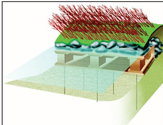
*Figure 4.5.11e Fish Lunker Structure Installed*
