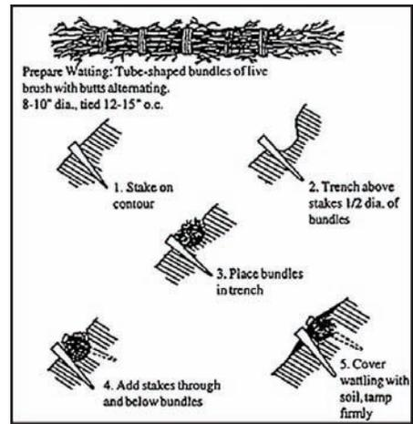
Figure 4.5.7c Installation of Contour Wattling
