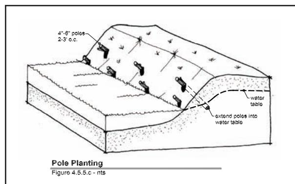
in constructed terraces or along existing contours of an eroding stream bank. When sprouted and rooted, the trees will stabilize the stream bank with a dense matrix of roots. This practice is usually applied to the splash and bank zones of a stream. Typically, a brush trench (see Practice 8) is installed at the top to filter overland flows. For severely eroded stream banks, toe protection such as log or rock revetment (see Practice 9) may be necessary. (Figure 4.5.6.a)
