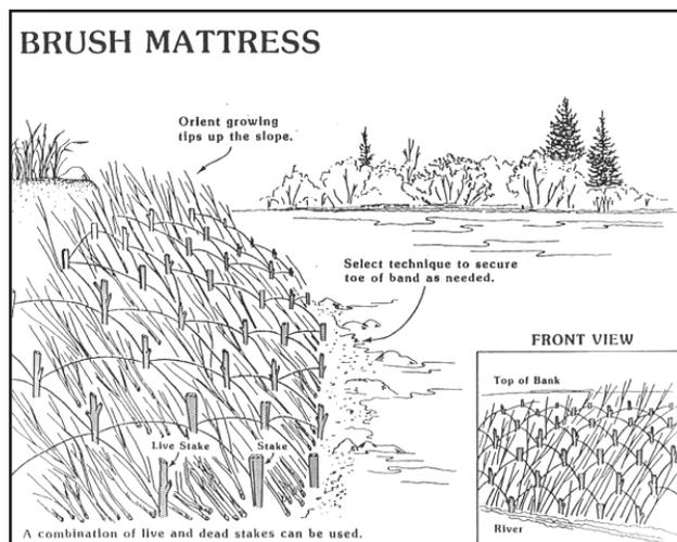
*Figure 4.5.7b Installation of Brush Mattresses
