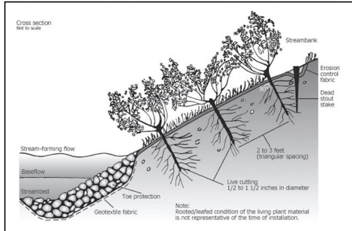
Figure 4.5.5b Installation of Pole Plantings
