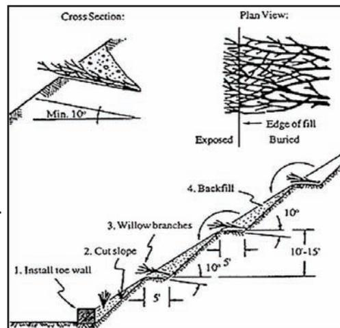
Figure 4.5.6b Installation of Brush Layering I
