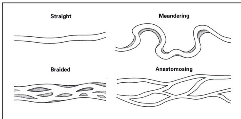
flow conditions. *Meandering* and *anastomosing* channels are common to the coastal plain of Georgia. The meandering river redefines itself by eroding the sediment on its outside curves and depositing the sediment on its inside curves, while the anastomosing river contains many separate channels that part and join again along its course.
