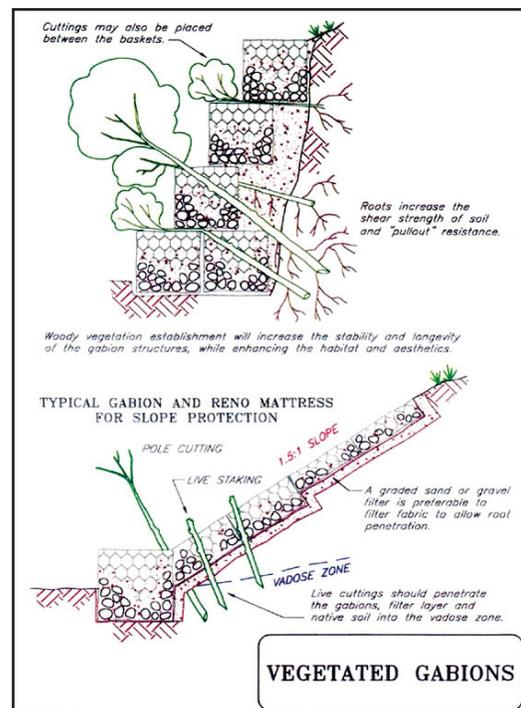
Figure 4.5.9e Installation of Vegetated Rock Gabions
