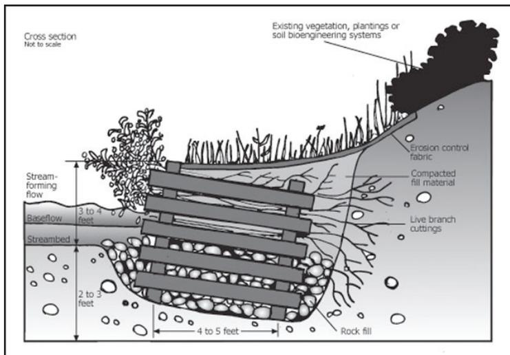
*Figure 4.5.10b Installation of Vegetated Cribwalls*
