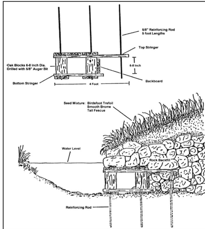
Figure 4.5.11g Installation of Fish Lunger Structure
