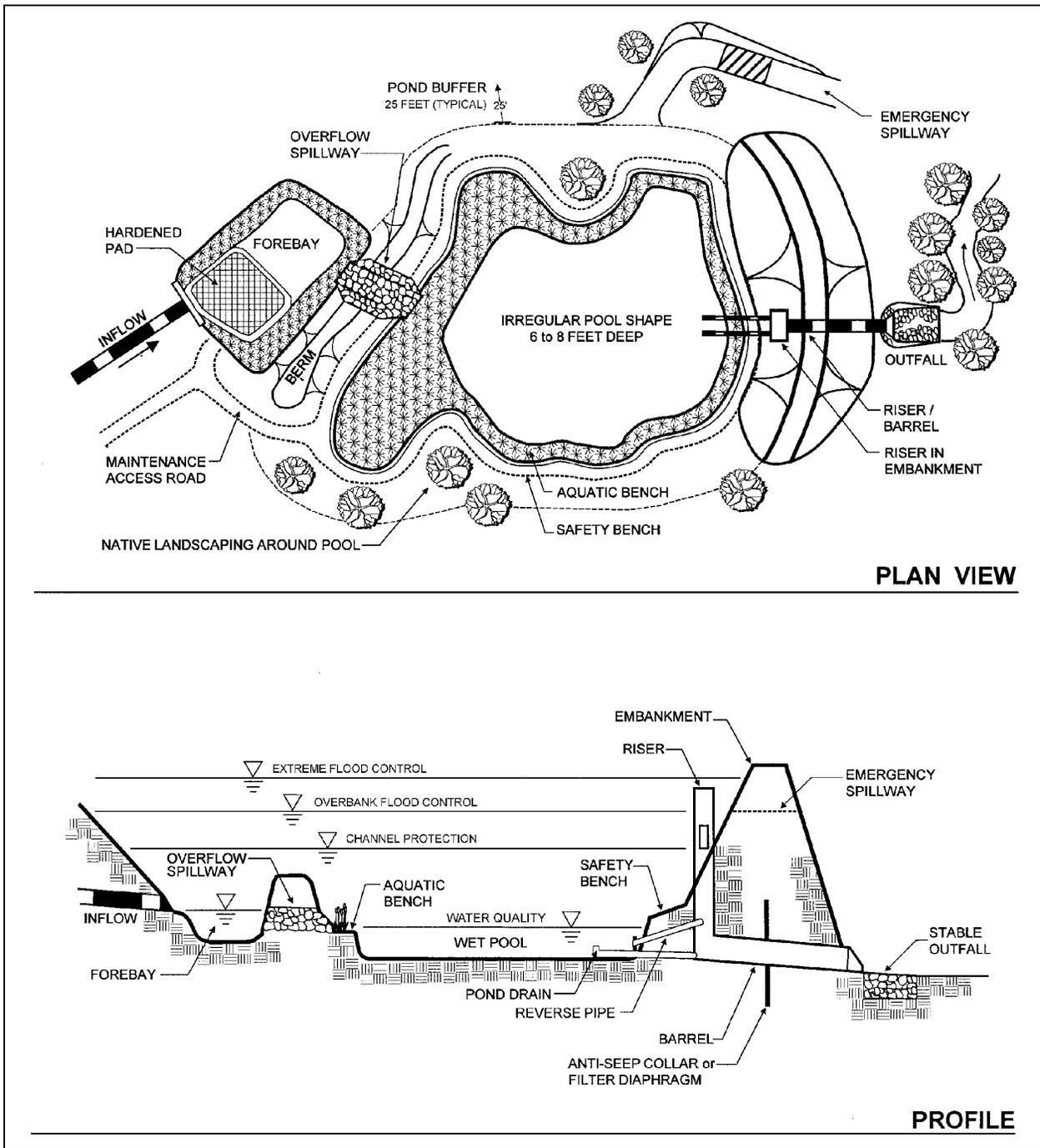
**Schematic of a Typical Wet Pond**
