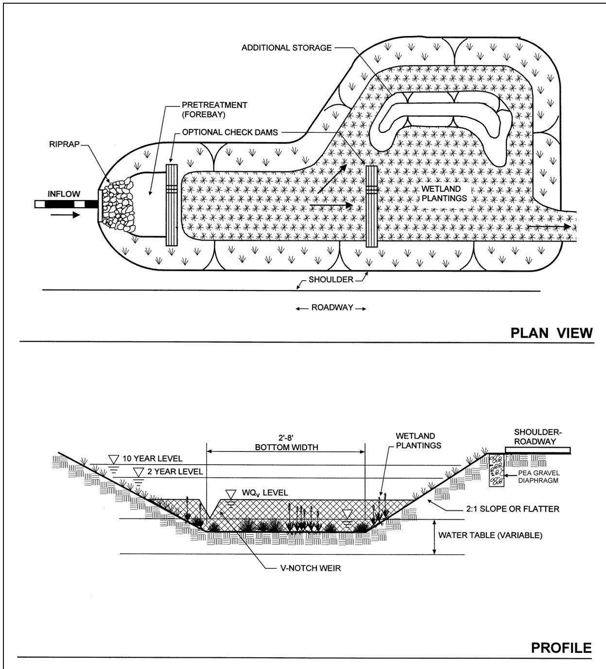
**Schematic of a Typical Wet Swale**
