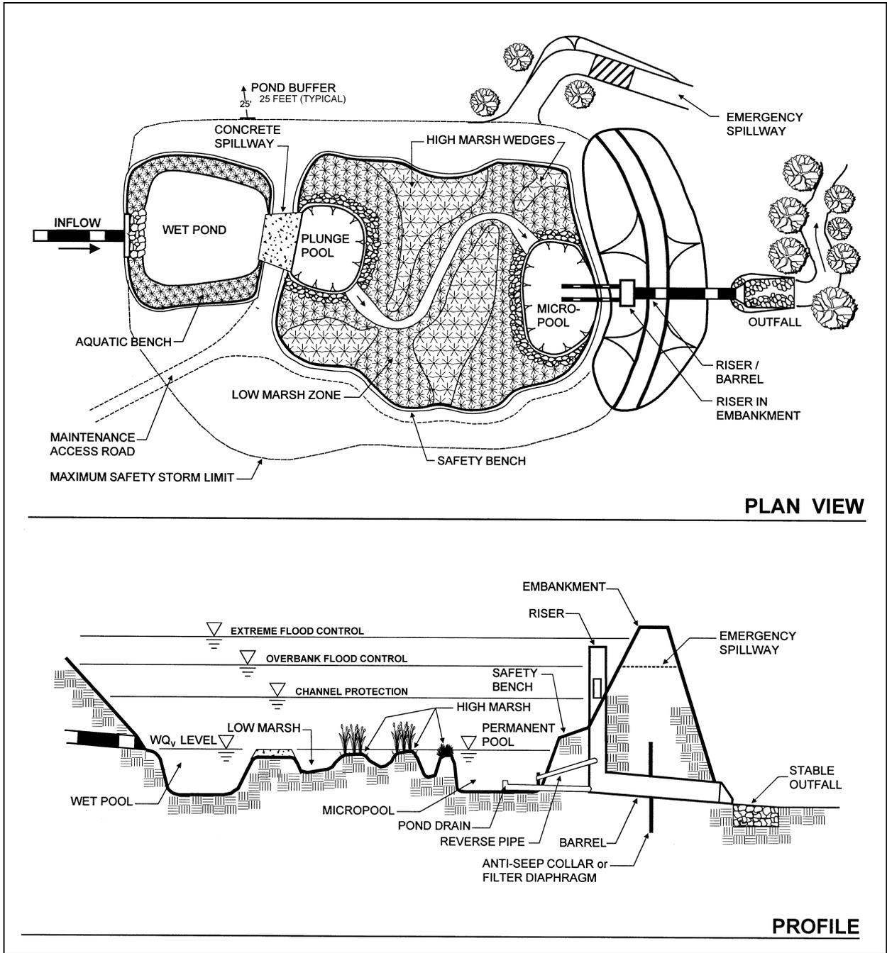
**Schematic of a Typical Pond/Wetland System**
