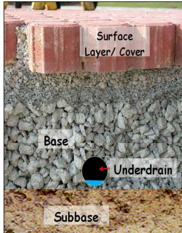
**Components of a Permeable Pavement System**
