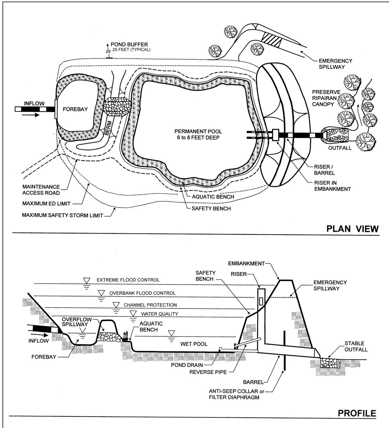
**Schematic of a Typical Wet Extended Detention Pond**
