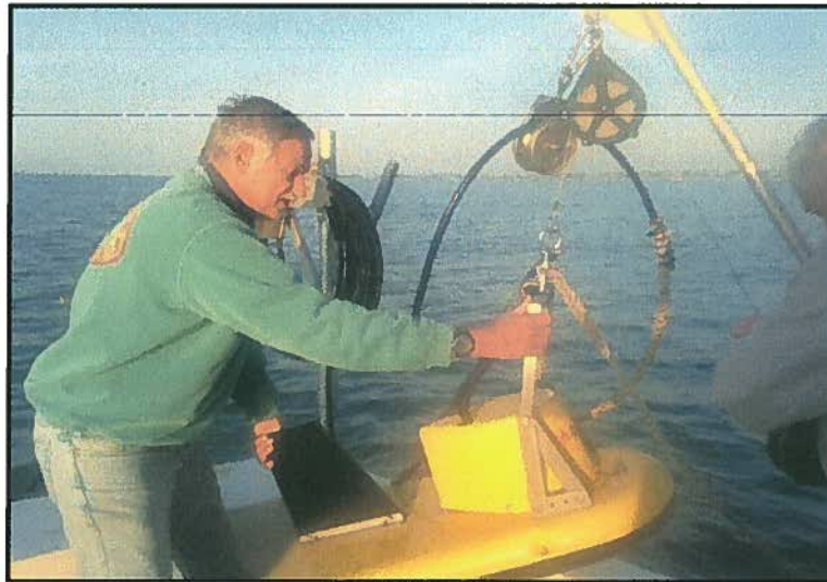
Figure 6. EdgeTech SB-216S tow vehicle.
