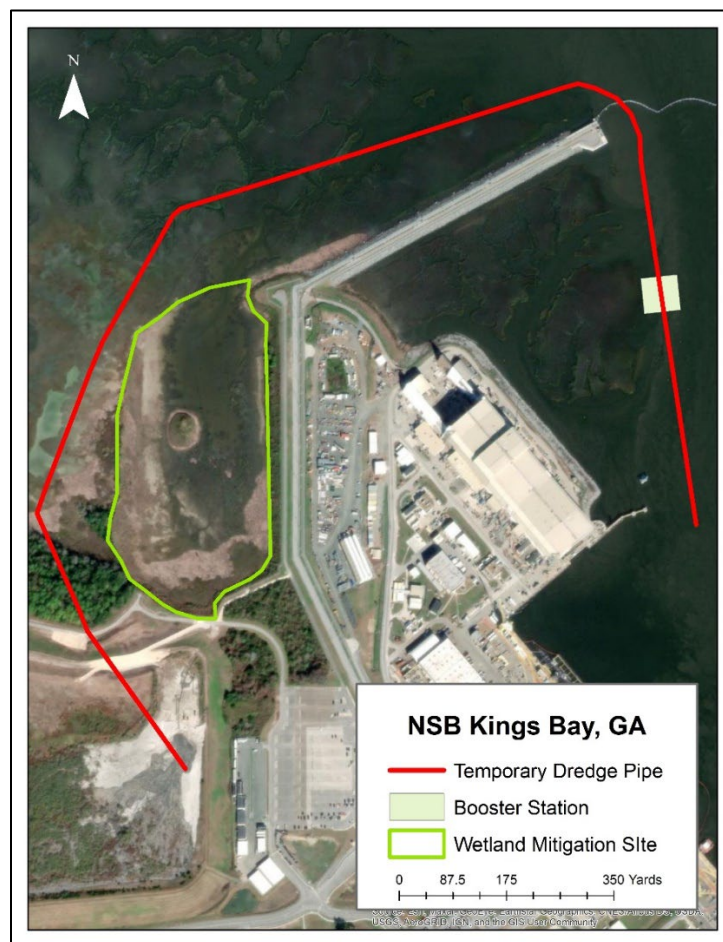
Figure 1. Proposed temporary (6 months) dredge pipe for disposal area 2 access during FY23 maintenance dredging operations.
