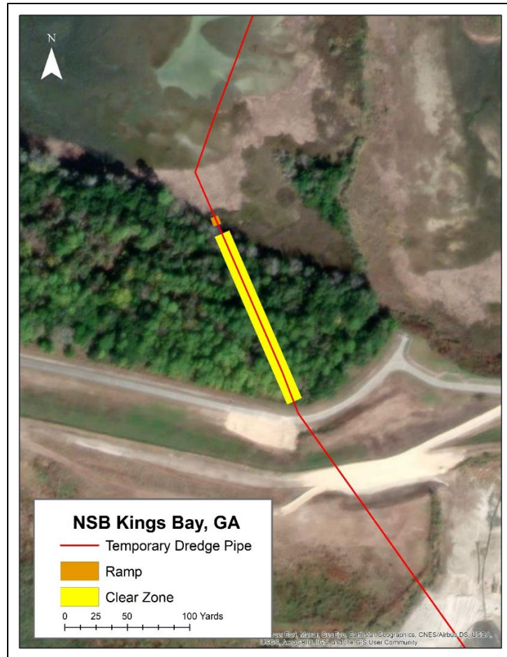
Figure 3. Upland areas traversed by proposed temporary (6 months) dredge pipe for disposal area 2 access during FY23 maintenance dredging operations.
