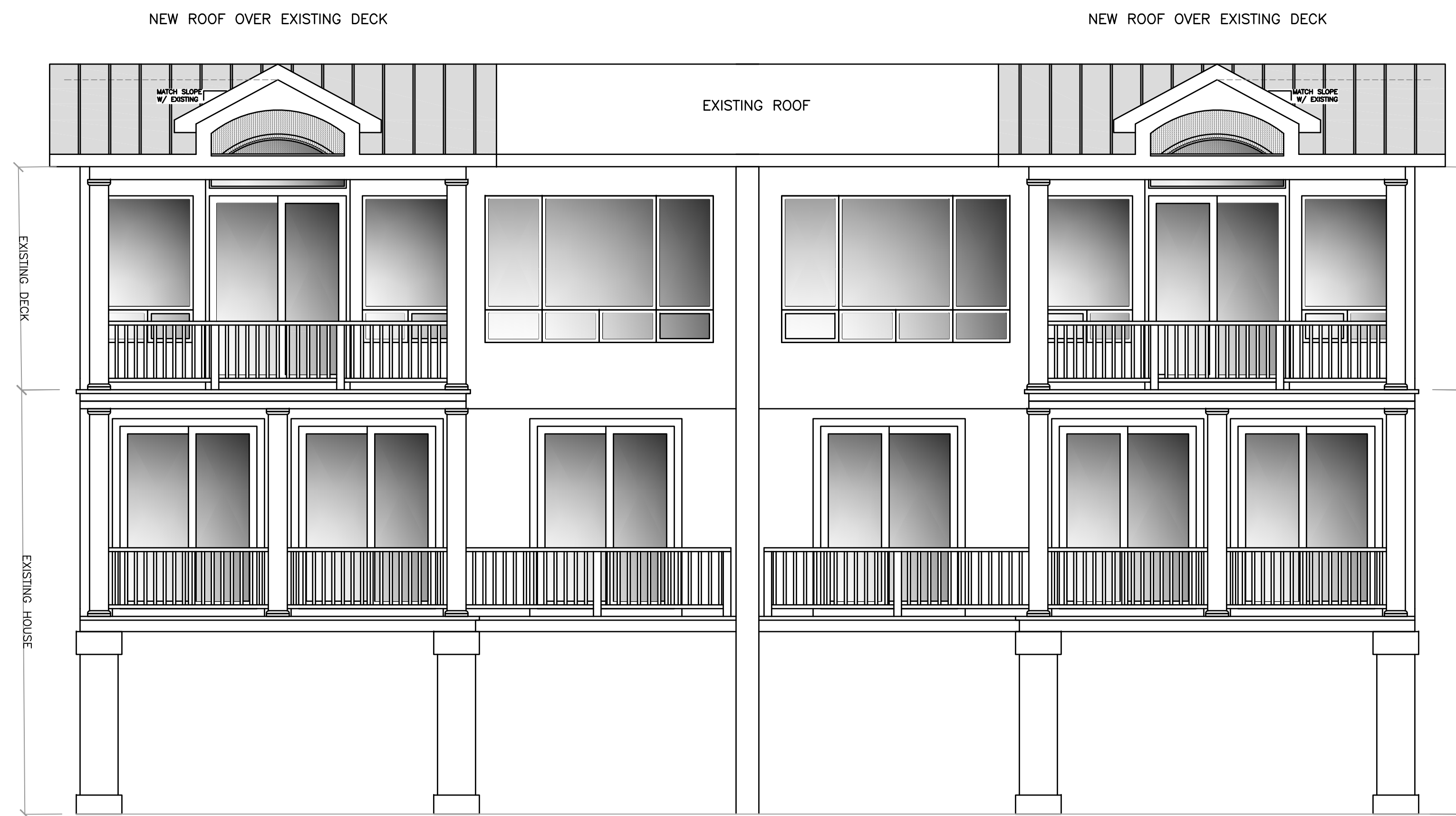
3 PROPOSED DECK ROOF ADDITION ELEVATION SCALE: 1/4" = 1' - 0"
