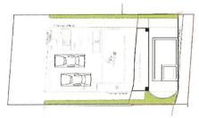
50 linear feet of 2" wide aluminum fence (64 LF x 2" = 9 square feet) will be constructed around the back yard.
