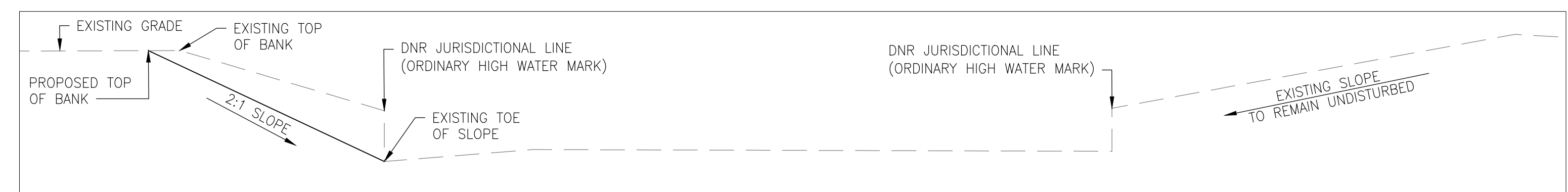
TYPICAL SECTION : OUTFALL DITCH
