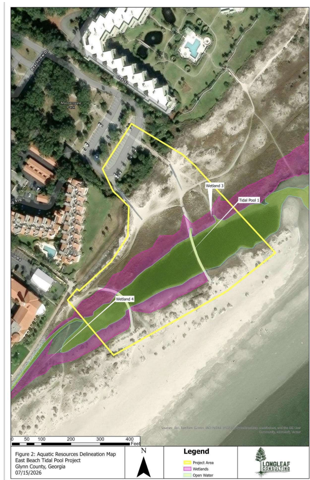
Figure 2: Aquatic resources delineation map with approximate boardwalk location. Wetlands and waters were field delineated using US Army Corps of Engineers (USACE) and state procedures in December 2025 and January 2026.
