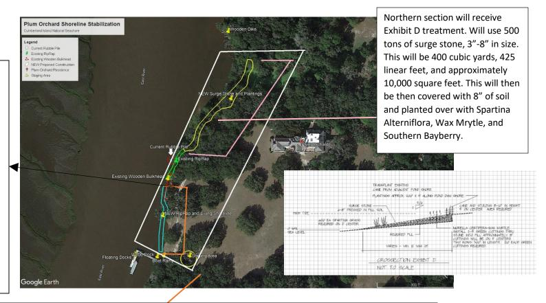
Southern section will receive treatments Exhibit C and Exhibit CI. Approximately 300 tons of riprap will be used the Exhibit C treatment. The length of impact is 214.29 cubic yards, 3716 square feet, and 225 linear feet. There will be approximately 5400 square feet of geotextile fabric placed below the riprap.
