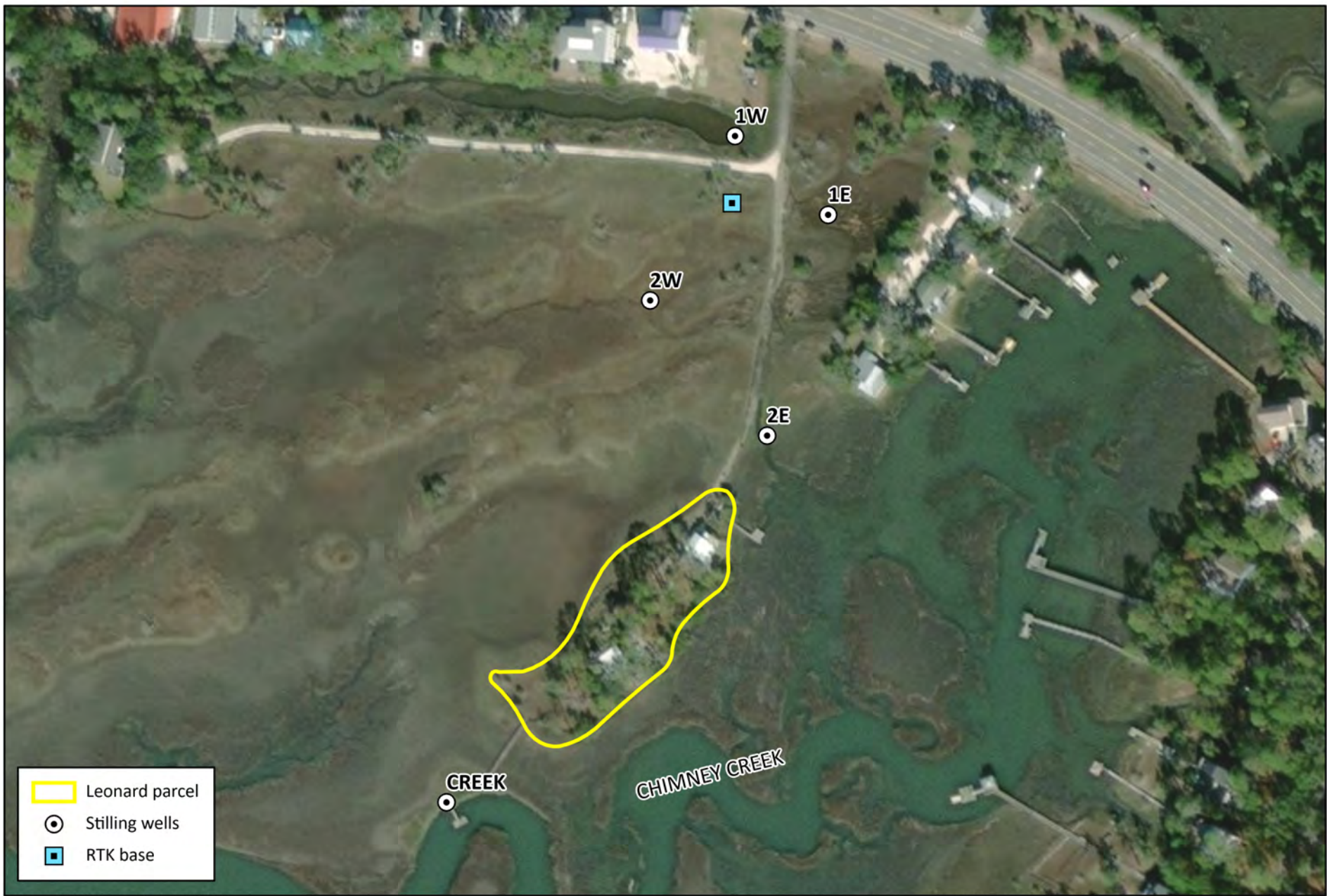
Figure 2. Stilling well locations and RTK base station within the vicinity of the Polk Street study area.
