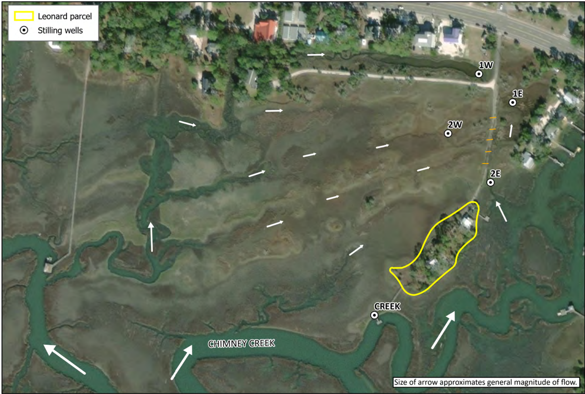
Figure 7. Primary water flowpaths into study area under current conditions. Orange arrows indicate areas where connectivity is limited to a small duration of time during high tide. Reference Figure 8 for more detail.
