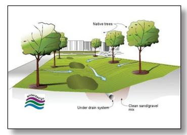
Figure 2.5b Bio-swale Schematic
