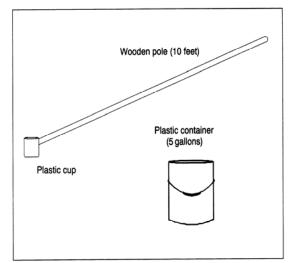
Figure 2. Liquid manure sampling device.
